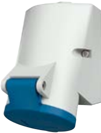
Wall mounted socket screwless, with TwinCONTACT, suitable for through wiring, internal fixing, 4 p and 5 p sockets the enclosure base can be turned 180°
