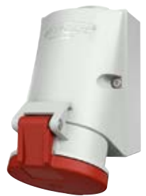
Wall mounted socket screwless, with TwinCONTACT, suitable for through wiring, internal fixing, enclosure base can be turned 180°
