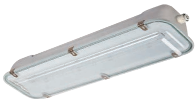
LED light fixture HT +55°C stainless steel-polycarbonate with comfort 88° extra wide beam optics IP66
