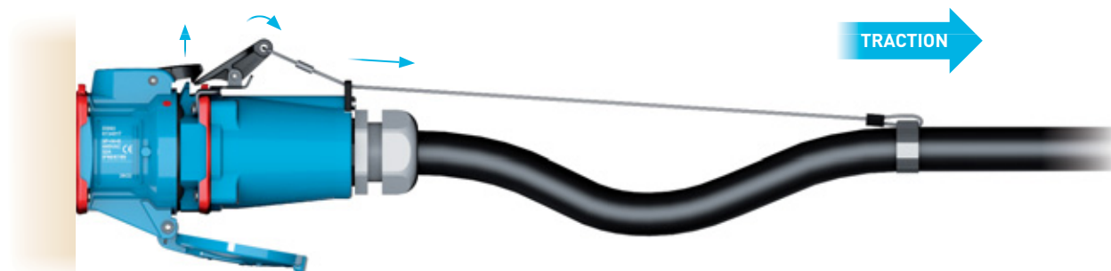
Step 2: the traction acts on the electrical cable and the rope. The ejection lever gradually raises the latch.
