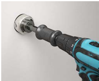
Create drill hole.
