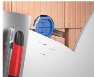
When plastering, the soft signal bristles wrap around without splashing and at a later time, indicate the position of the box.
