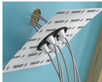
Before the sleeve can be glued in position, make sure that the surface is free of dust. Then remove the protective foil,...
