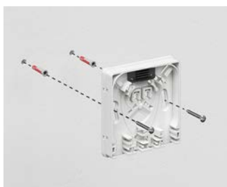
Create 5 mm drill holes.
