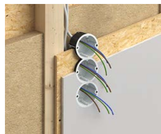
...in an F60-B wall, individual boxes up to a 3 box combination are possible.
